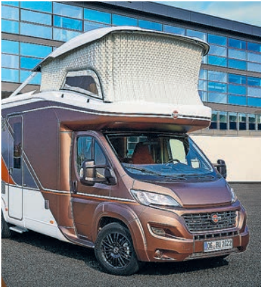
While travelling, the Bürstner Lyseo Gallery is partially integrated but, having arrived at its destination, it is an alcove model.
