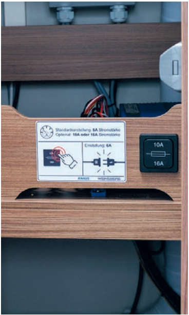
A few of the Südwind and Sport models by Knaus are already available with E-power. Depending on the amps available at the campsite, you can switch to 10 or 16 amps.
