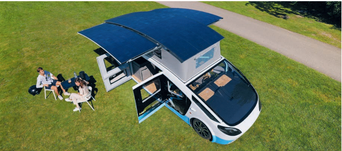
The Stella Vita has a top speed of 120 kilometres an hour and, on a sunny day, can go up to 730 kilometres.
